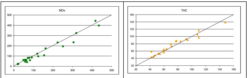
*Figure 2: comparison between measured and predicted  $\text{NO}_x$  and THC emission levels*
