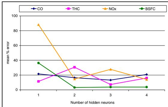
*Figure 1: effect of the number of hidden neurons on the mean % error for CO, THC,  $\text{NO}_x$  and BSFC prediction*
