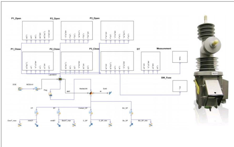
Figure 2: modeFRONTIER workflow piloting the Hardware-In-the-Loop (HIL) process
