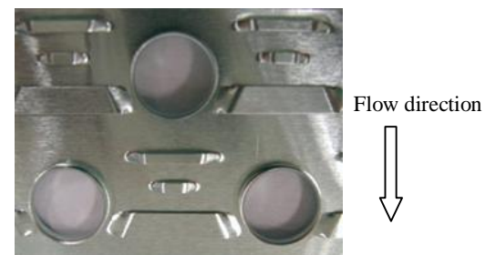
Fig.9 Fin shape determined by optimization.
