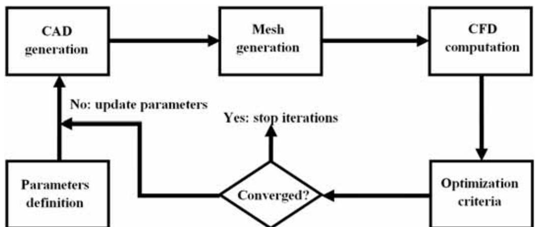
Fig. 1 - Flow chart of the optimization procedure.
