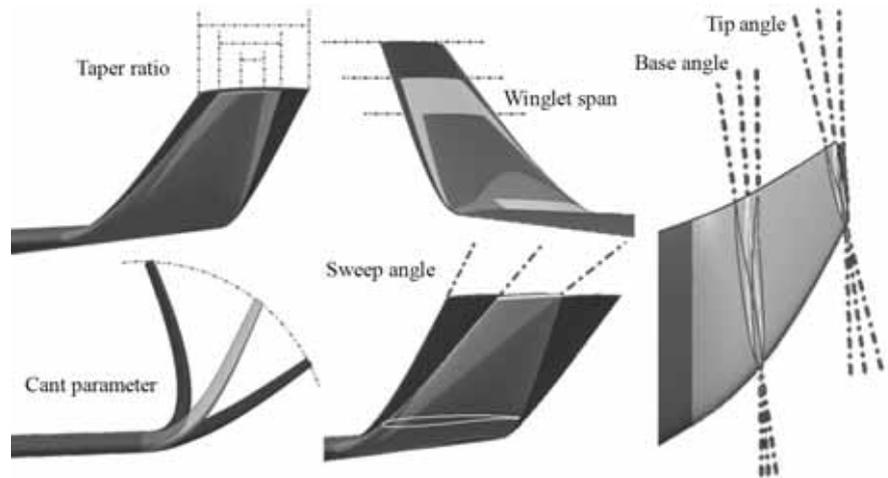
Fig.2 - Winglets CAD model and design parameters.
