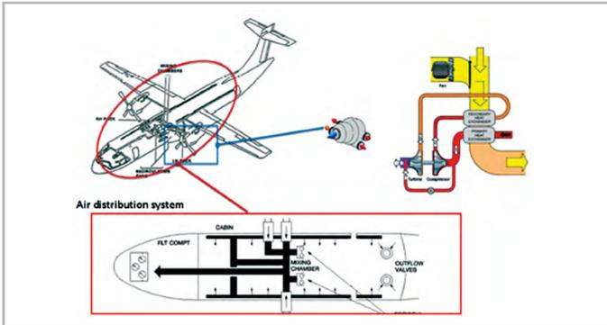
Air flows from the engine processor and through the air conditioning pack before distribution.
